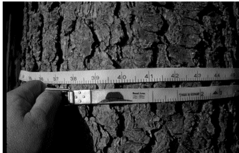
Using the MTG tape to measure Tree Diameter at Breast Height Over Bark. The DBHOB of this tree is 41.1cm.
