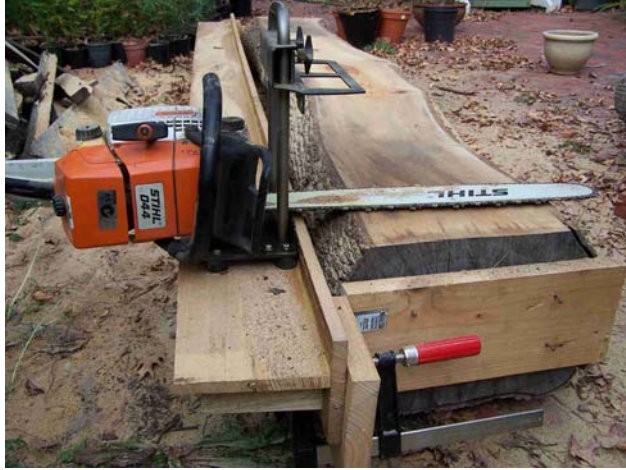
1372: The first cut: the timber guide is fixed in place using two end brackets
