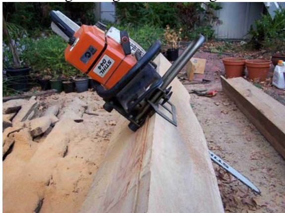
1374: The timber guide can then be removed and successive boards cut off using the dimension plate. The plate can be easily adjusted out to about 20cm.
