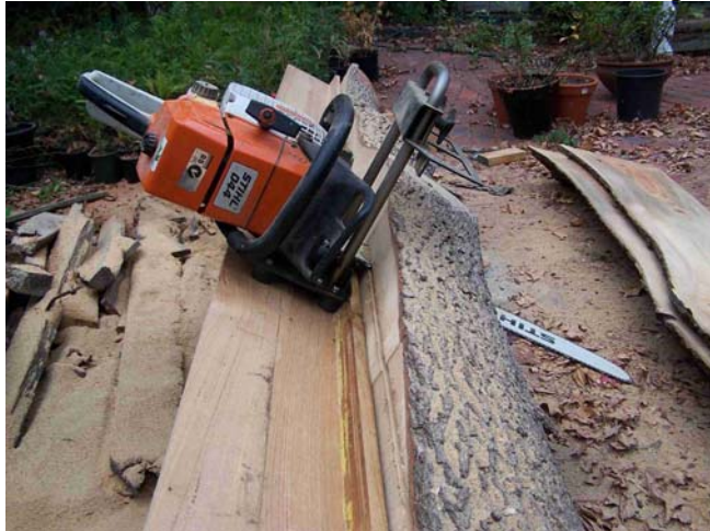
1373: The second cut: the guide is put against the clean face to produce a right angle cut. Tilting the log makes holding the saw in place a little easier.
